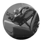
Image: Wedge ejecting during crash test
